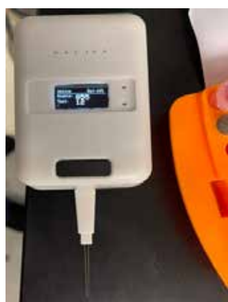
Fig. 6.3a: Photographic image of P-FAB device (10x6x3 cms) with the probe cartridge (6x1 cm) and a U-bent fiber optic probe. b. A proof-of-concept for N-protein detection (down to sub-ng/mL) using the sensor with a standard reference from ICMR (Courtesy: VoxturBio, Mumbai) obtained using the lab set-up.
