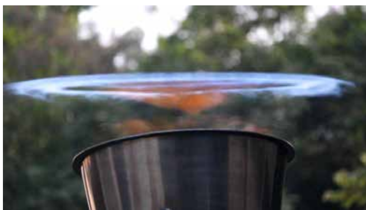
Fig. 5.1: Detonation wave obtained with LPG/air mixture at \phi = 1.2
