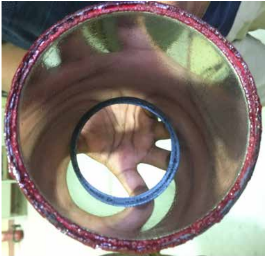
Fig. 3.89: Automotive engine cylinder bore coated with Ni alloy
